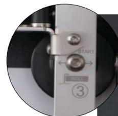
The beginning of the metal profile is in line with the middle of third roll marker
